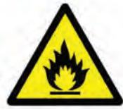
Flammable material or high temperature
